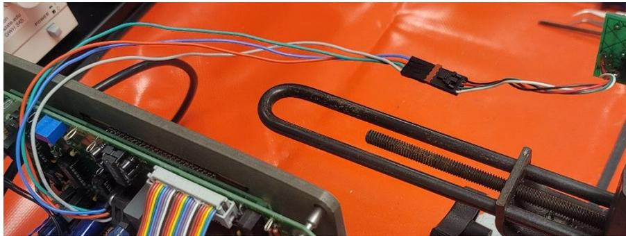
10. Connect the Laser Board to the CPC using the extension cable. Attach a scope probe to TP1 (yellow circle in Figure 9). There is a ground post as shown.
