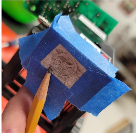
7. Place painter's tape over the laser board's exposed solder side circuitry facing the optics block to avoid shorting traces during adjustment.
