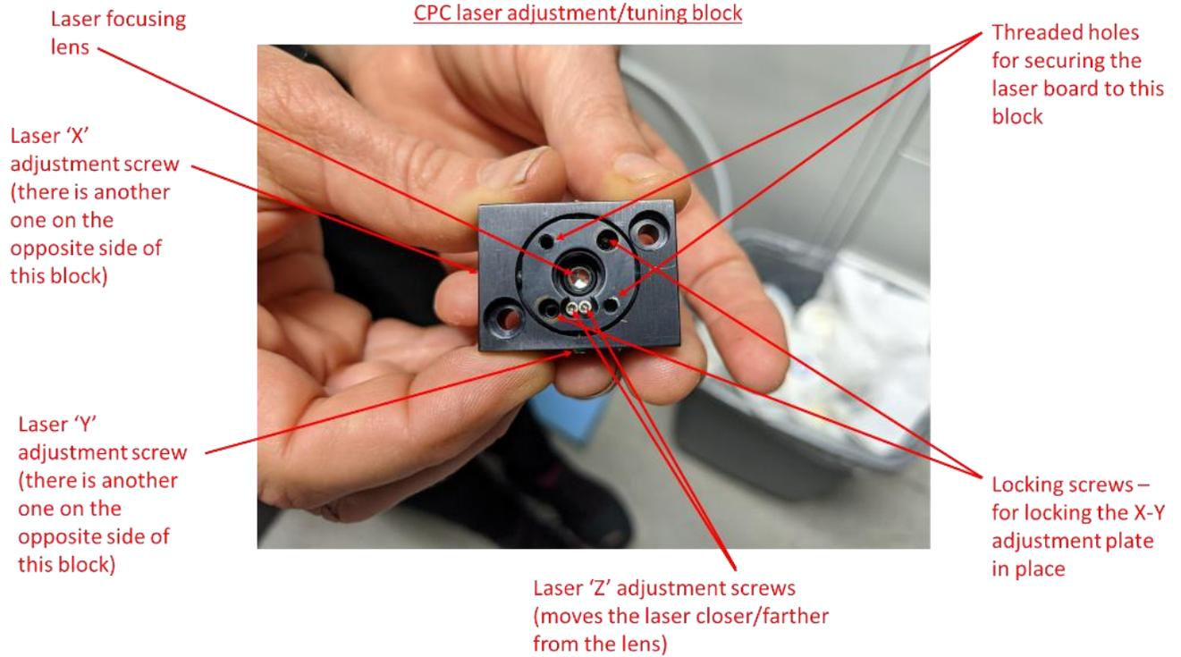
Figure 12. Optics Block Setup with X direction hex keys in place
