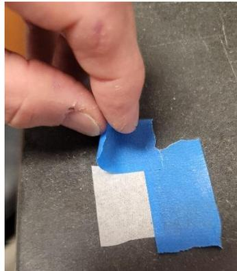
5. Pull the screen up and affix it over the center of the optics block detector hole.
