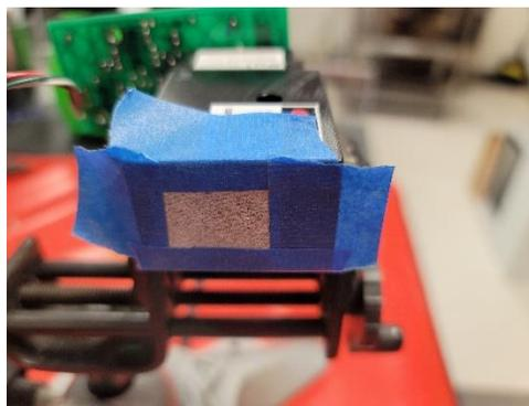
6. Using a standard pencil, make a rubbing to exactly outline the detector opening
