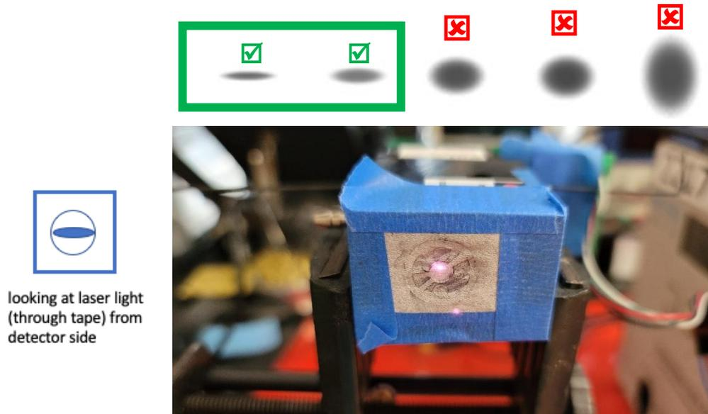
4. Once you have the beam centered in the X direction, tighten both 'X' screws. You may need to make fine adjustments until you get it spot on.
