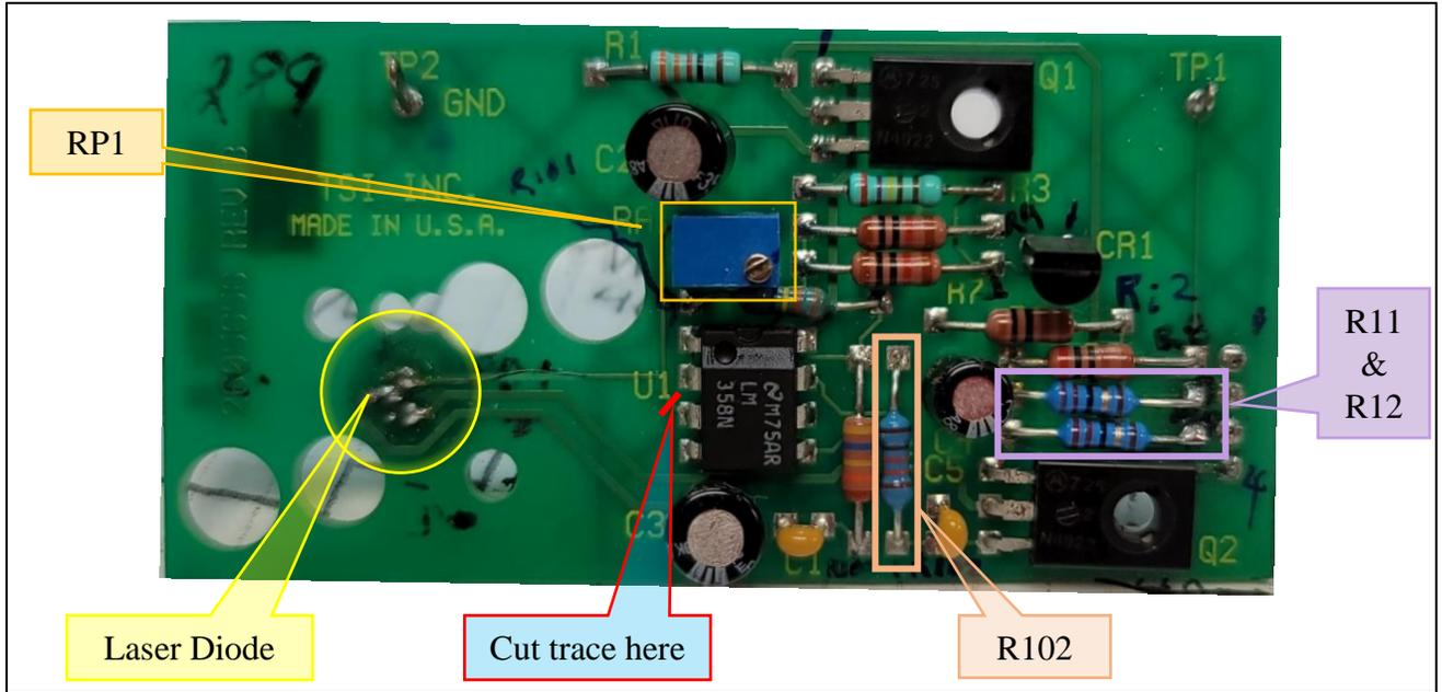
Figure 6. Solder Side Rework
