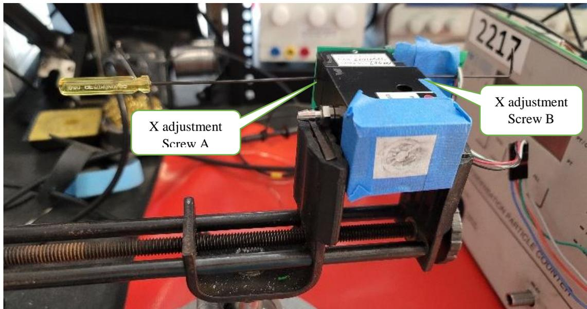
1. Referencing Laser Adjustment / Tuning Block in Figure 11 on page 14, loosen the two 5/64" X-Y locking screws 1/8 turn. Loosen more if you must for adjustment, but the less free play the better.
