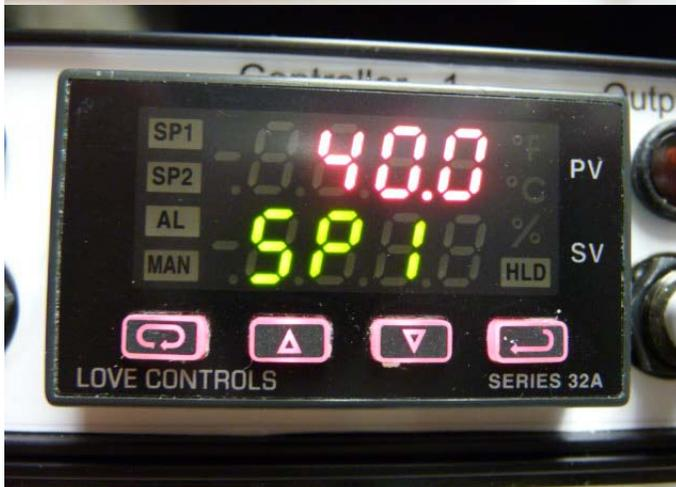
This is where you adjust the set point. Press UP or DOWN arrows to adjust. Press Enter to retain value. Here the top red number is the desired setpoint.
