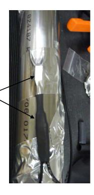
Thermal cutoff switch goes in middle of pipe. (note: heater in this picture is old version – cord heater)
