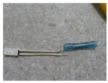
Triple fold skinny wires on thermal cutoff switch for better crimp.
