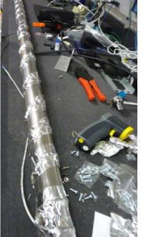
Attach heater to pipe using foil tape. (Careful – the tape has got sharp edges!)
