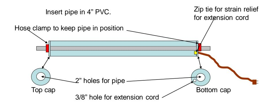
No need to glue together, although could glue top cap if desired.
