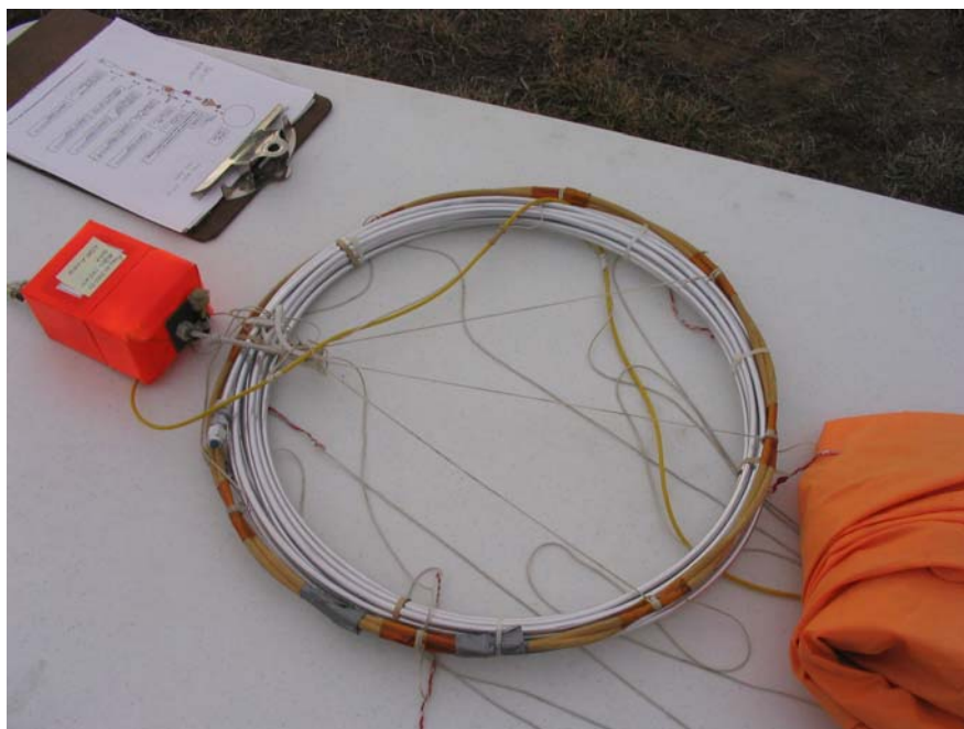
Figure 1. View of the AirCore flown by balloon to an altitude of 80,000 ft (24,384 m) on February 26, 2005. The Aircore in this case is 15-m length of aluminum tubing. The portion of the parachute is in the lower right corner, and the cut-away fuse is in the box on the left.
