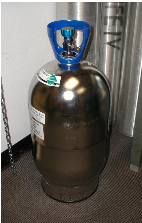
Figure 1. Electropolished 34-L stainless steel cylinder used to develop water vapor standards.
