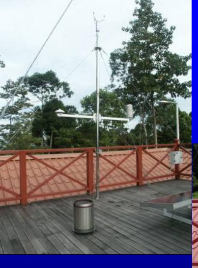
Vaisala AWS and Ecotech wet-only collector (precipitation chemistry)
