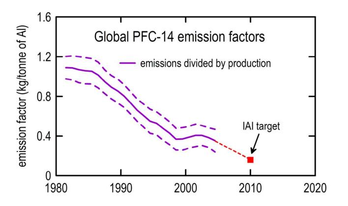
1980s emission factor 1.1 kg PFC per tonne of AI
