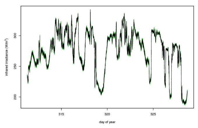
**Figure 1.** Multiple determinations of downwelling infrared irradiance over 17 days in November near Boulder, Colorado, using all 92 determinations of the calibration constants determined in the GMD blackbody.
