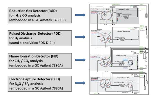
Figure 1. Setup and parallel operation of the GC trace gas analysis line.
