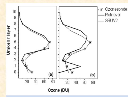
Test  $O_3$  profile retrieval (sza=75°) for GSFC (a) for the real atmosphere with aerosols and (b) neglecting aerosols with a pure Rayleigh atmosphere. The SBUV2  $O_3$  profile (grey) and the ozonesonde results (\*) are shown in comparison to the retrieval (black).
