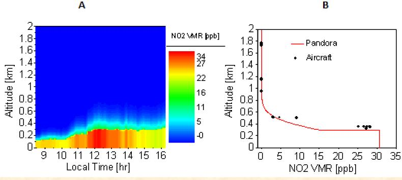
NO<sub>2</sub> profiles derived from Pandora direct-sun and MAXDOAS observations over Fresno, California on 18-Jan-2013 Comparison of Pandora retrieval to aircraft (P3B) measured NO<sub>2</sub> profile (Fresno California).
