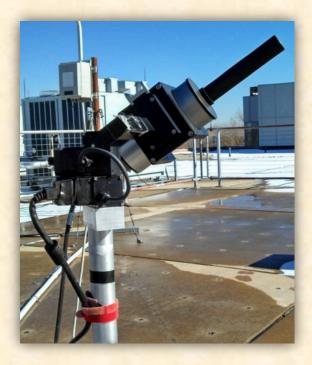
The "Detector" connected by optic cable to an optical head (1.6° field of view) mounted on a high precision (0.01°) sun-sky tracker.
