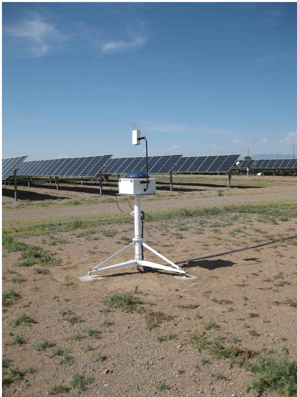
**Figure 1.** Total Sky Imager at an Xcel Energy Utility Plant, Colorado
