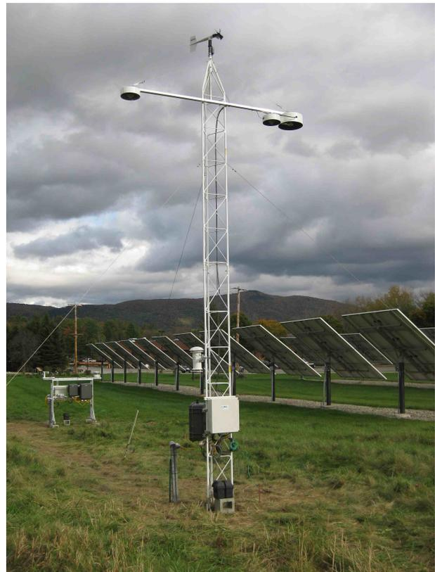
**Figure 2.** Mobile SURFRAD installation in Rutland, VT with Green Mountain Power
