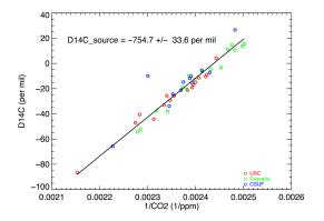
**Figure 1.** "Keeling Plot" of November, 2014 through January, 2015 CO<sub>2</sub> and <sup>14</sup>CO<sub>2</sub> data from three sites in the Los Angeles Basin. The D<sup>14</sup>C\_source value (the y-intercept of the regression) for purely fossil fuel-CO<sub>2</sub> additions to background would be -1000 per mil; the less negative source signature of -750 per mil indicates additions of sources with isotopic ratios close to that of the atmosphere (i.e. ~ 0 per mil).
