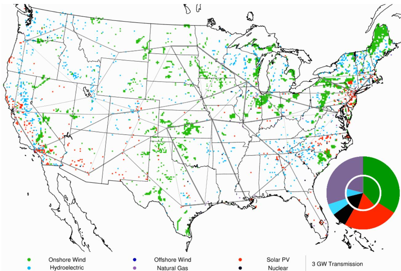
**Figure 1.** A cost-optimized single electric power system for the contiguous U.S.. The colors indicate that a model grid cell has a technology sited within it. The gray lines show the HVDC transmission network. The outer pie chart on the right represents the installed capacity by technology, while the inner pie chart shows the electric demand met by each technology. Electricity is shared across the entire U.S. along HVDC transmission lines connected to 32 nodes.
