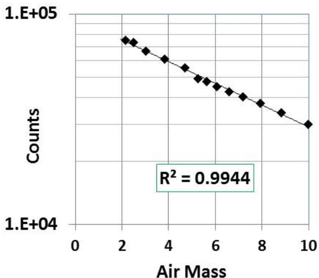
**Figure 2.** Langley plot using the star Rigel in Orion under very low aerosol conditions. The R2 of 0.9944 is equivalent to an AOD error of about 0.02.
