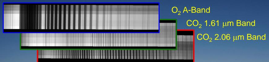
Each 1/3 of a second frame includes 8 spatial footprints with 1,016 wavelengths sampled in the  $O_2A$ -band and Weak and Strong  $CO_2$  bands
