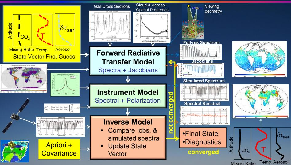
GOSAT Data have provided a critical validation of the OCO-2 Algorithm
