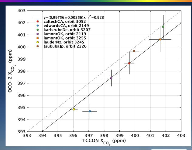
**Comparisons with Total Carbon Column Observing Network** (TCCON) stations are being used to identify and correct biases in target observations. (Wunch et al.) **Initial differences** between OCO-2 and TCCON X<sub>CO2</sub> estimates were smaller than ~2 ppm (0.5%).
