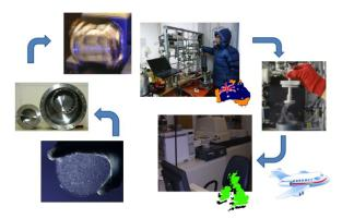
Figure 1. Air trapped in bubbles in glacial ice is extracted with a shaken "cheesegrater" device and collected in cold-fingers at ~10K at the CSIRO-CMAR laboratories in Melbourne, Australia, and subsequently analysed at UEA in Norwich, UK with a gas chromatograph/tri-sector mass spectrometer combination.
