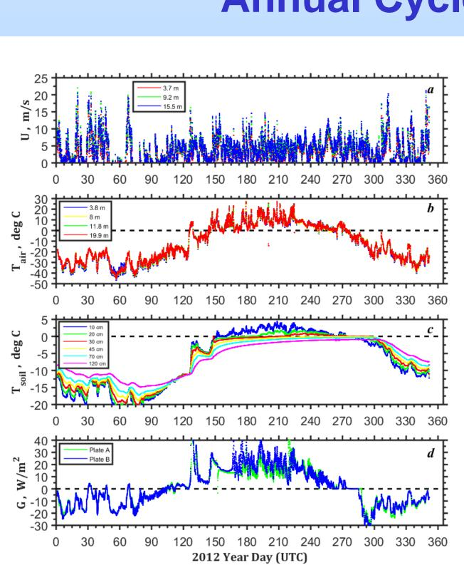
Annual cycle of (a) wind speed at 3.7, 9.2, 15.5 m (wind vanes), (b) air temperature at 3.8, 8, 11.8, 19.9 m (RTD sensors), (c) soil temperature at 10, 20, 30, 45, 70, and 120 cm, (d) soil heat flux (plates A and B) observed at Tiksi in 2012. The data are based on 1-hour averaging.
