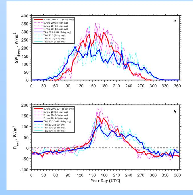
Annual cycle of the solar radiation at the 'top' of the Annual cycle of (a) short-wave (SW) downwelling radiation and (b) net radiation observed at Eureka in 2009-2011 and Tiksi in 2012-2014. The net radiation in the bottom panel is defined as the balance between incoming (positive quantity) and outgoing (negative quantity) SW and LW radiation. The data are based on 5-day averaging of 1-hr radiation measurements.
