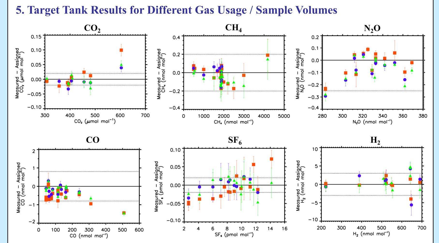
Sample gas usage: 325 mL vs. 525 mL on Magicc-1 Measurement over larger mole fraction ranges Efficient operator interface and dual sample manifolds improve capacity
